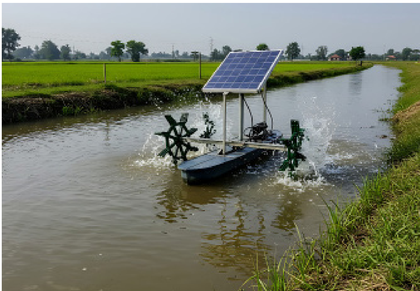
solar energy powered waterwheel aerator
